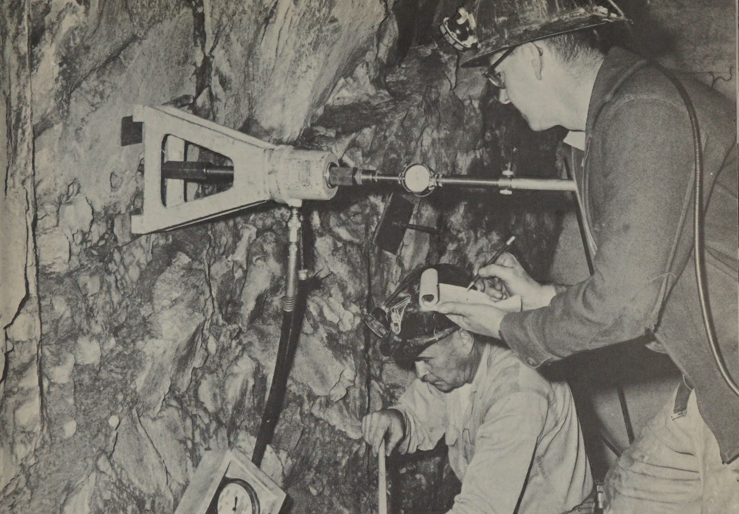
These Bureau of Mines engineers in the Coeur d'Alene District conduct a pull test on a new Bureau-developed device.
